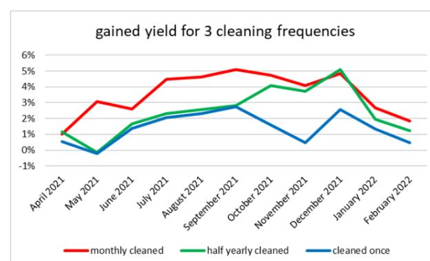
Regular cleaning of EnTranCe' PV panels resulted in a small gain in production, this effect is less when cleaning is less frequent.
