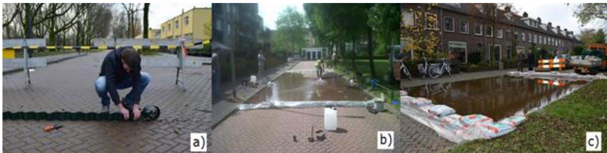
**Figure 3** Various Dam Variations Used at the Different Test Locations (a) Impermeable barriers; (b) Plastic wrapped soil core; (c) Soil-filled plastic bags.
