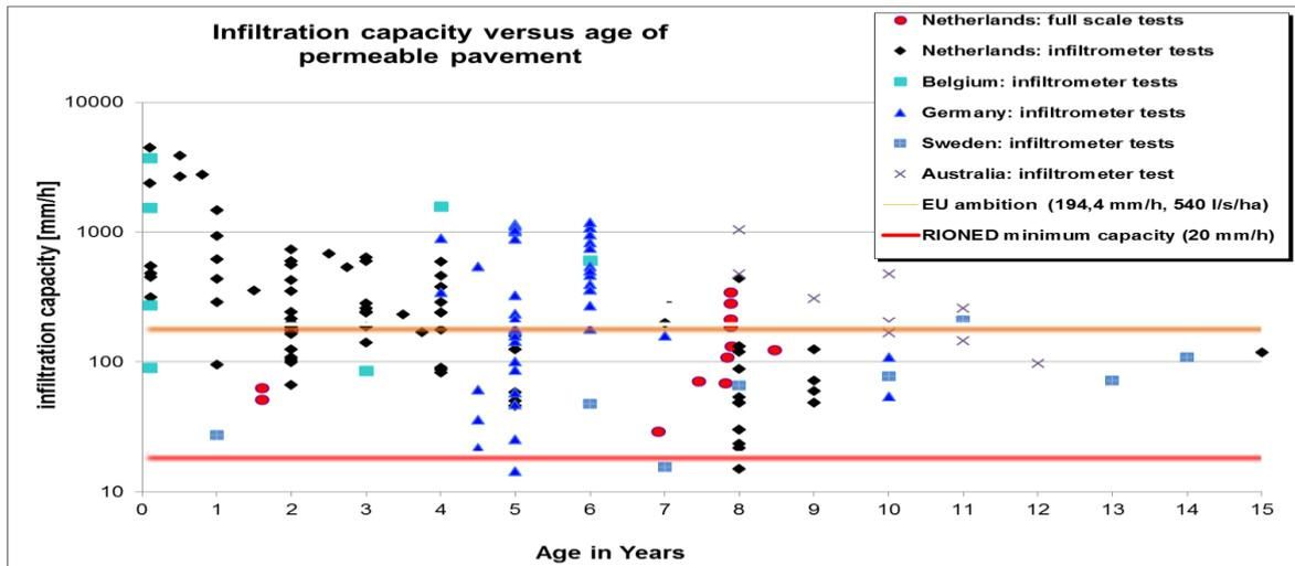
**Figure 5** International permeable pavement infiltration capacity research results [Boogaard, 2015]
