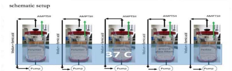
Figure 2: different carriers (polymer 1 and 2, sand, ground glass filters and perlite) are tested in a small batch reactor. In each reactor, MTA medium is pumped around with formic acid (2 grams / liter). Hydrogenotrophic methanogens convert formic acid to CO<sub>2</sub> and CH<sub>4</sub>. Both the CO<sub>2</sub>, the CH<sub>4</sub> and the formic acid concentration are measured.
