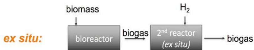
Figure 1. Reactor set-up used for biological methanation
