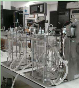
**Figure 4: Two Infors 13 liter Labscale Bioreactors:**
