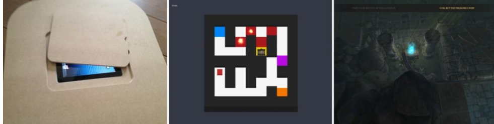
Fig. 1. Impression of the game setup; from left to right: (a) the balance board with an iPad embedded; (b) an early 2D-prototype of the maze navigation game and (c) a screenshot of a further elaborated 3D version of the game.
